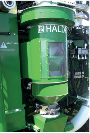
POLYTEC NIR spectrometer system on a HALDRUP C-65 plot combine
