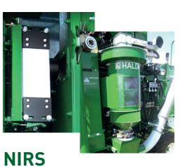
Near infrared spectroscopy
